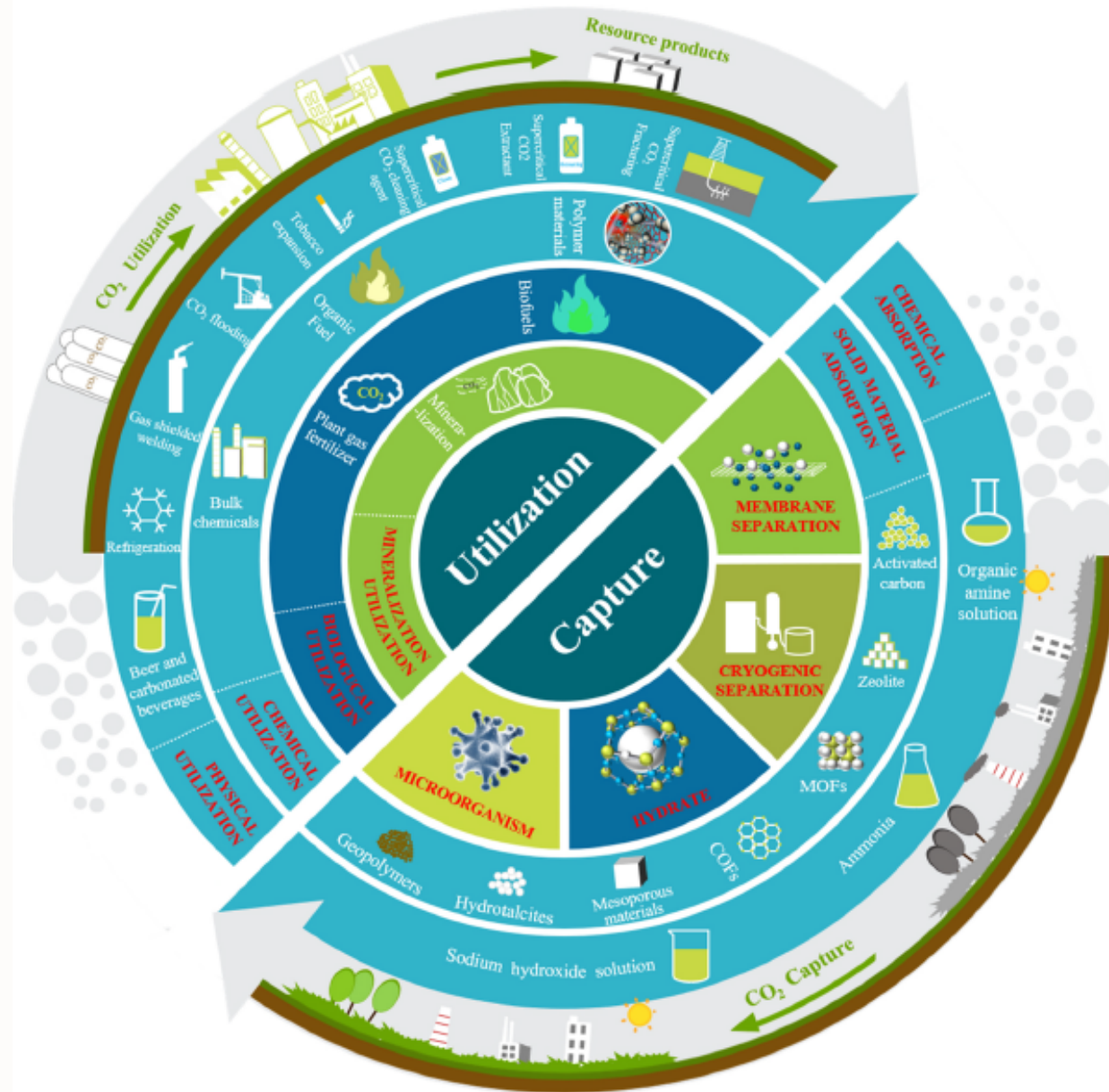
Fig. 1. Schematic diagram of CO 2 capture and utilization cycle.
