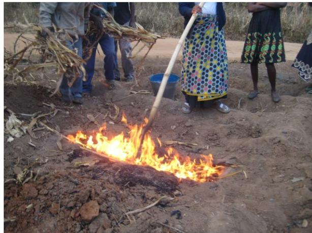
Training to make biochar in flame cap pit kiln. No smoke.
