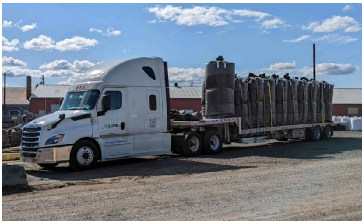
Step deck flatbed truck loaded with 19 pallets of 4 yards 76 cubic yards of biochar on board. Biochar Solutions LTD.
