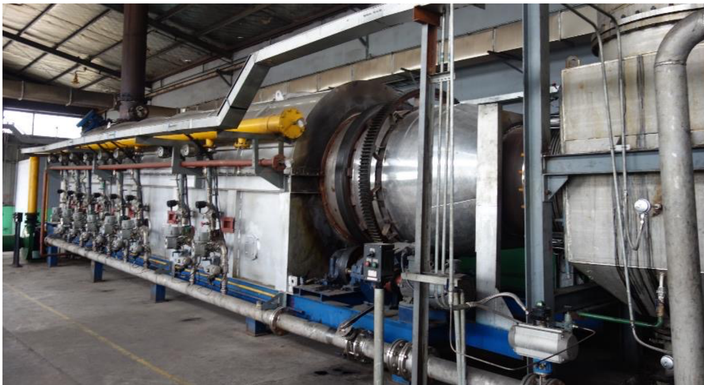
Sanju Crop Residue to Biochar Fertilizer Production Facility 2.5 mt/hr, gas+pyrogas
