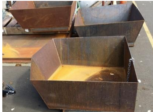
UCC Welding program made heavy duty kilns with fork pockets for easy moving with a tractor or fork lift. One kiln has a spout and tilt mechanism for dumping.
