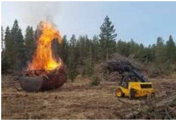
Arborist Brandon Baron makes biochar in a modified 10,000-gallon water tank and a shipping container (Photo: The Tree Service, Burns, Oregon).
