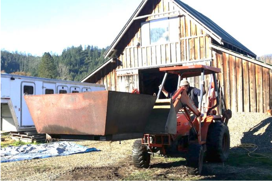
Using the kiln with fork pockets at Page Creek Ranch.
