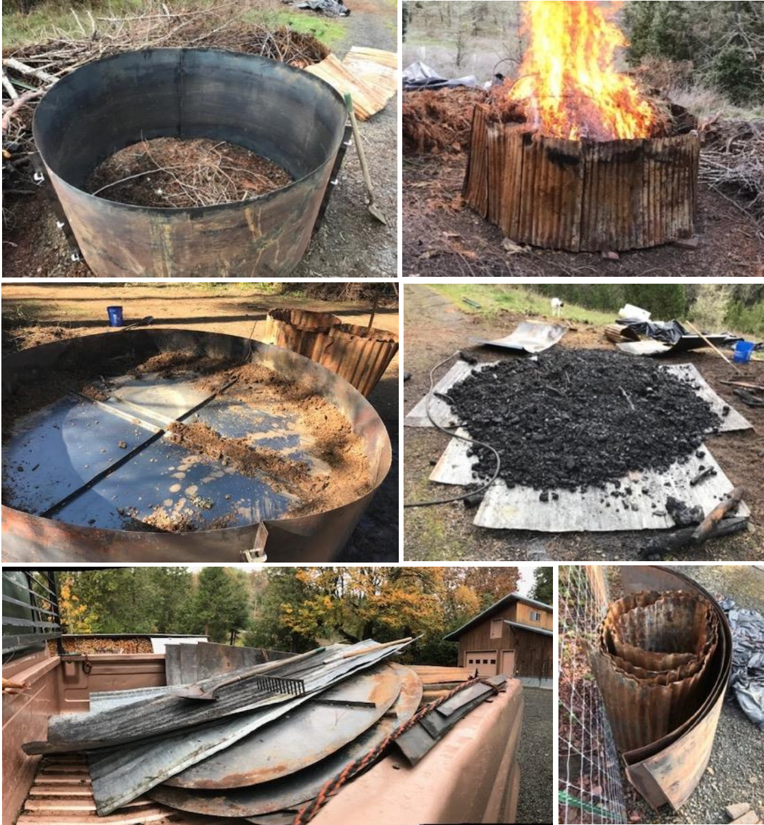
Ring of Fire Kiln showing kiln assembly; outer ring set up on blocks for air flow; quenching lid sealed with dirt; finished biochar; components disassembled for transport.
