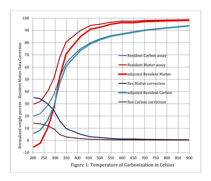
As can be seen in the trends in Figure 1, any biochar that has been produced at temperatures below 240C has no adjusted Resident Matter and negligible adjusted Resident Carbon. All biochars produced below 400C have significant corrections associated with the high level of volatiles and the associated correction being applied to generate the adjusted Resident Matter and Carbon metrics. Above 400C, and
