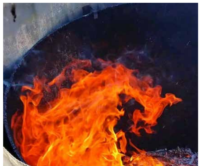
Flame tips curl downward in a flame cap kiln, showing how all the air comes from above in a counter-current flow. Photo by Kelpie Wilson.
