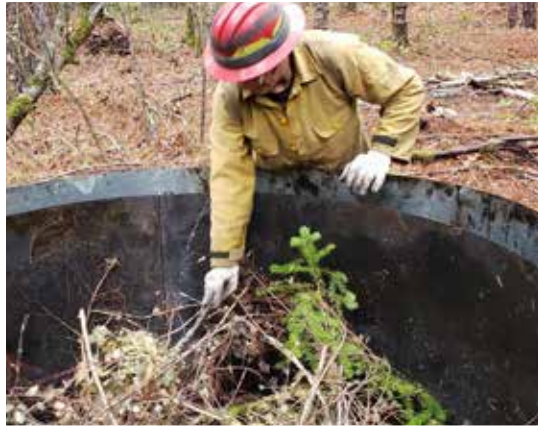
Load. Load the initial feedstock, keeping it loosely packed.
