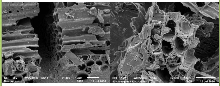
Images of Mesquite and Mesquite/Juniper Mix Biochar made using a TSI torreactor
