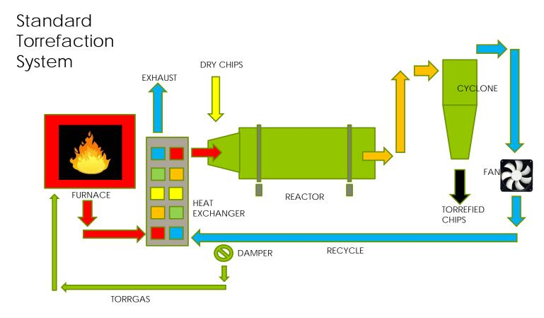
The TSI reactor heats via a heat exchanger and is auto-thermal.
