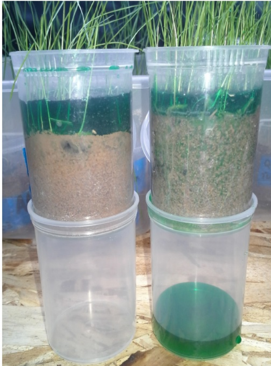
Figure 17. Infiltration comparison between QEP control and Biochar (5 tons/acre), green dye is used to illustrate flow paths through soil profile
