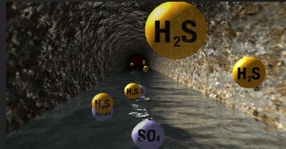
H_2S generated from sulfates in waste water
