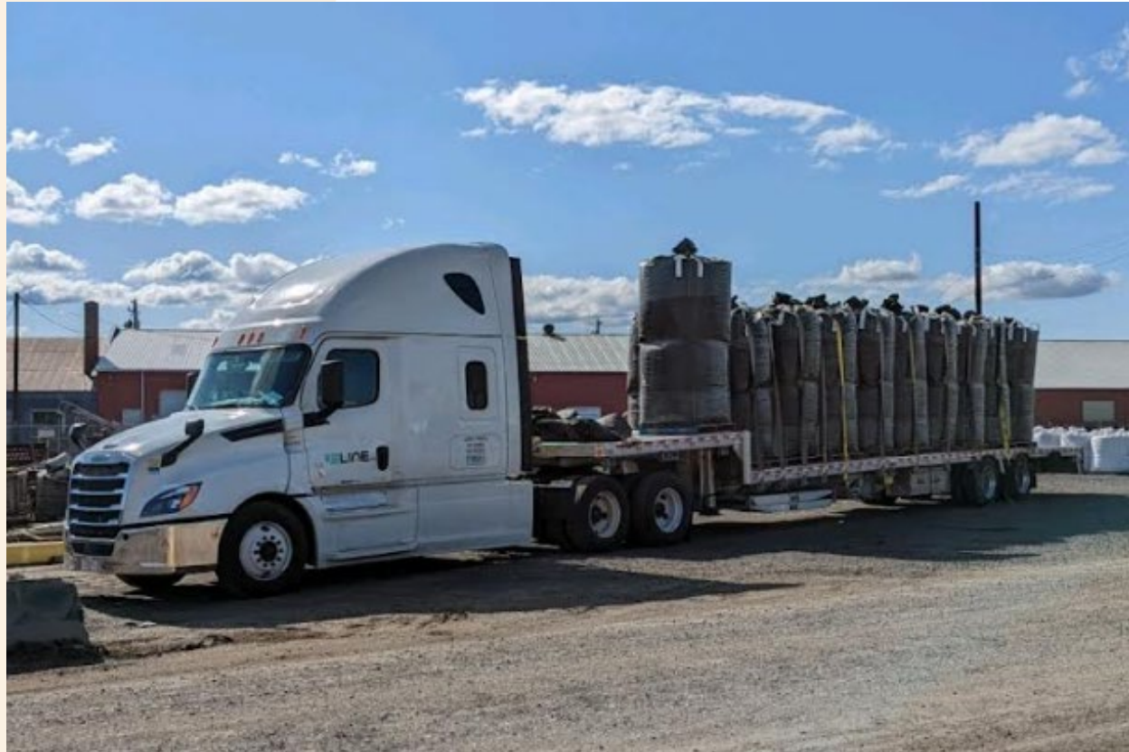
A step deck flatbed truck loaded with 19 pallet of 4 yards – 76 cubic yards of biochar on board. Biochar Solutions LTD.
