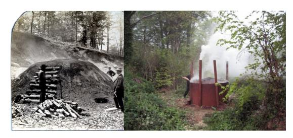
Capturing Energy — Today, biochar is produced using pyrolysis, that is, biomass is super-heated in the absence of oxygen at high temperatures (350-700°C) in specially designed furnaces. The most sustainable feedstocks is are what's now considered waste: excess manure, wood debris, construction waste, slash from forest thinning, food processing waste, residue from methane digesters or urban tree trimmings. Most of this would be left to rot, be open-burned or dumped in a land fill.
